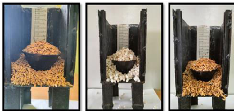
Figure.3 Thermal conductivity of paddy, popped rice, husk through thermal analyser
